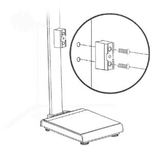
Use the 2 screws for screwing the bracket into the supplied insert nuts on the stand of the scales.
