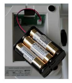
⇒ Insert battery holder with the inserted batteries into the display unit
